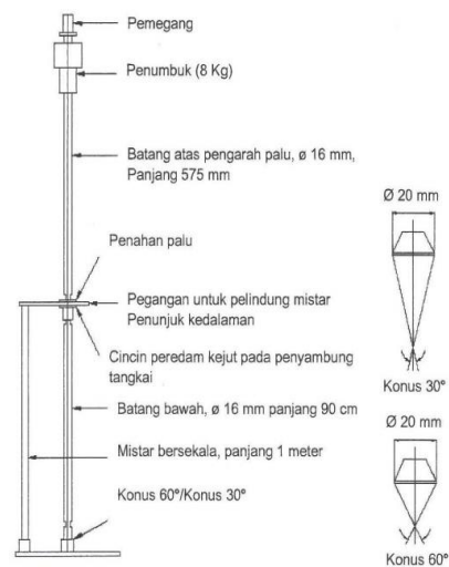
Gambar 2. Alat Dynamic Cone Penetrometer (DCP) [12]
