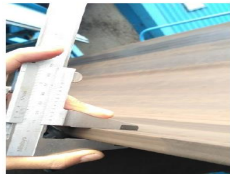
Gambar 3. Mengukur ketebalan belt conveyor
