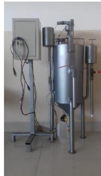
Gambar 3 Prototype Continius Settling Tank
